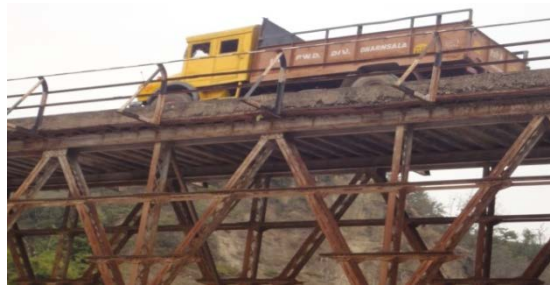
Fig.5 Truck placed to measure deflection
